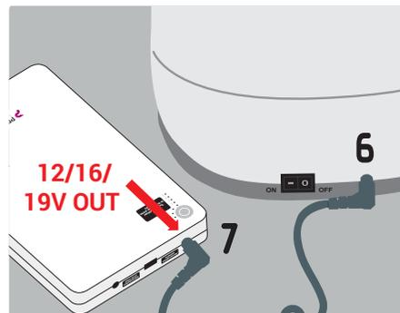
Connect the C2S Pro system to the battery with the provided cable. Then connect the cable to the battery on the output «12/16/19V OUT». **The C2S Pro system is now autonomous.**
