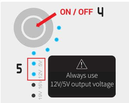
Turn on the battery by a long press on the button ON/OFF then check if it's on the position 12V/5V. If this is not the case, press the button twice to change the output voltage. Repeat until 12V/5V is reached.
