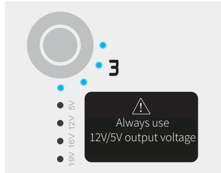
When charging the battery, the blue LEDs blink. The battery is fully charged when all LEDs are fixed and lit.
