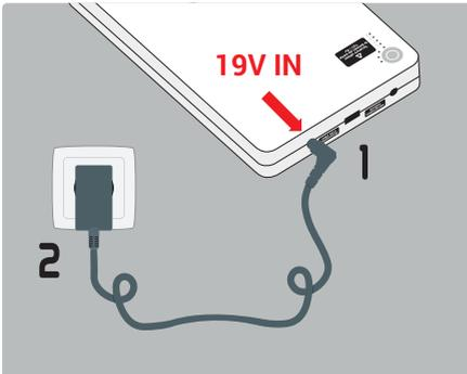
Connect the supplied standard adapter to the «19V IN» port of the battery supply. Connect the charging plug to your electrical installation.
